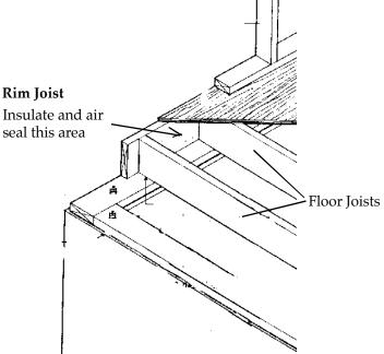
**Figure 6:** Cut-away view of top of basement wall, looking down from first floor
